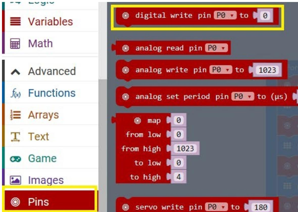
Figure 6. Digital write block in the Pins drawer
