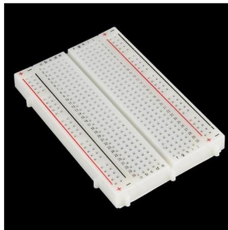
Figure 3. Breadboard for prototyping circuits
